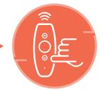
8. Press and hold the DOWN button to test that the motor direction is correct.
